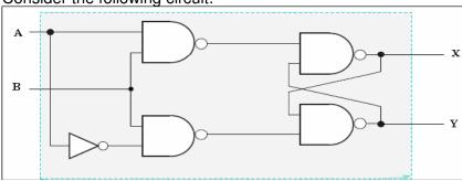
Assuming that initially X = 0 and Y = 1, show the waveforms for X and Y if the following inputs are applied:
